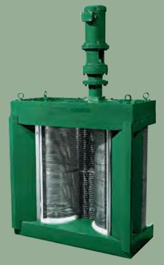
Channel Monster® sewage grinders are designed to capture and grind down the toughest wastewater solids in high-flow systems. Common applications include protecting pumps in lift stations and grinding up solids at the plant's headworks.
