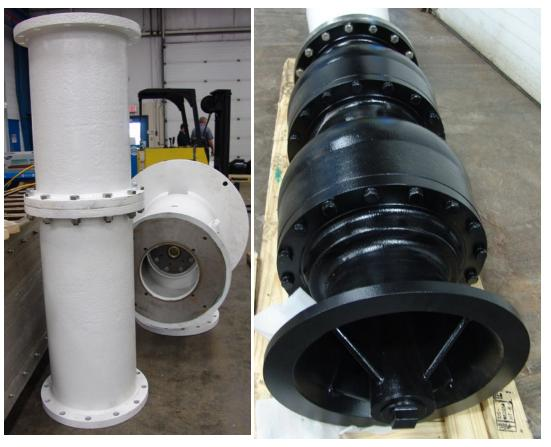
Rebuilt discharge head and flanged columns (left) and bowl assembly (above).
