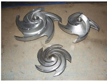
Examples of open vane impellers.
