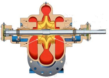
Inside of a double suction split case pump. Arrows point to inlet eyes on the impellers.
