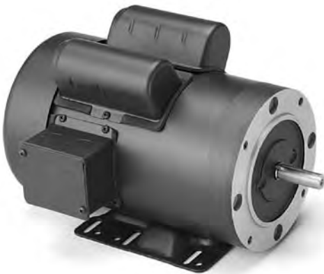
On industrial duty motors, capacitors are usually protected by metal cases attached to the motor frame. This capacitor start/capacitor run motor has two cases.
