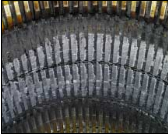
Figure 19. A major core rub; not repairable unless core is dismantled and repaired.
