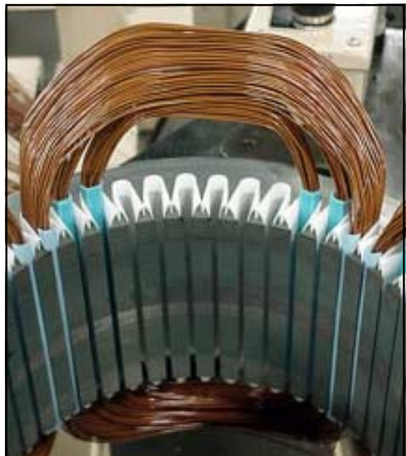
Figure 35. In a concentric winding, each coil has a different span. Each span has a different chord factor, making the effectiveness of each coil different.
