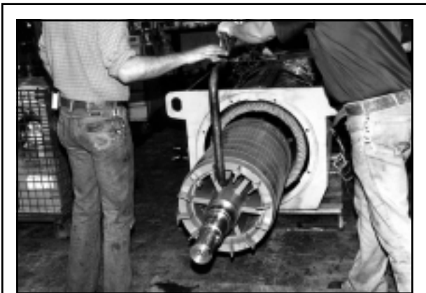
Figure 17. Rotor removal using a rotor removal tool.
